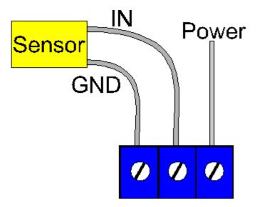
When measuring 4-20 mA with the EL037 supplying loop current, the transmitter should be connected like this:
