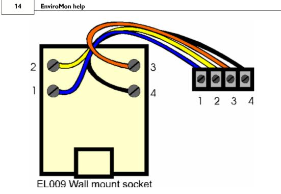
Connect adjacent units using four core cable, eg WI003. Connect terminal 1 to terminal 1, terminal 2 to terminal 2, and so on. The following table shows the signals associated with each connection:
