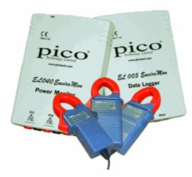
The current monitoring kit provides a complete solution to measuring three channels of mains current. This could typically be applied to measuring and balancing three-phase supplies or monitoring the increase / decrease in current drawn from mechanical equipment to aid maintenence schedules.
