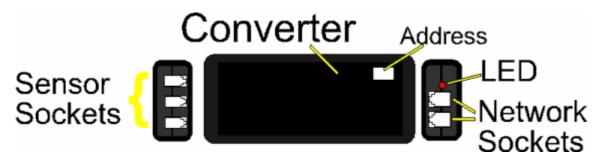
The LED flashes continuously immediately after the system is turned on. Once the system is running normally, the light goes out and, thereafter, flashes briefly each time the converter takes a reading.
