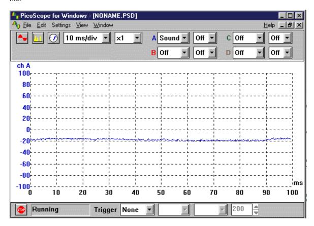
Try clicking your fingers over the microphone: the trace on the screen should react. DrDAQ is now successfully installed and working.
