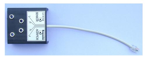
The range of Auto Detect and Signal Input voltage must be between 0 and 2.5 volts. This is a hardware limitation and any signals outside of this range will not be read by the unit. Any voltages greater than +/- 30 volts fed directly into the device are likely to damage the unit, and can cause errors with all other DrDAQ readings.
