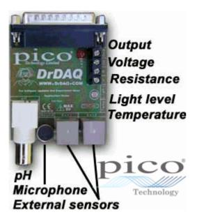
DrDAQ is a low-cost data logger from Pico Technology. It is supplied ready to use with all cables, software and examples. Features include:
